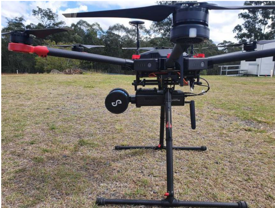
Figure 8 HF1 Autonomous Waypoint mode: Forward mounting
