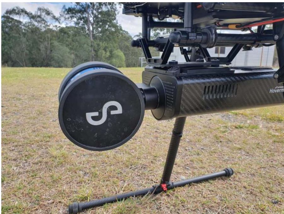
Figure 7 Autonomous Waypoint mode: Forward mounting close up
