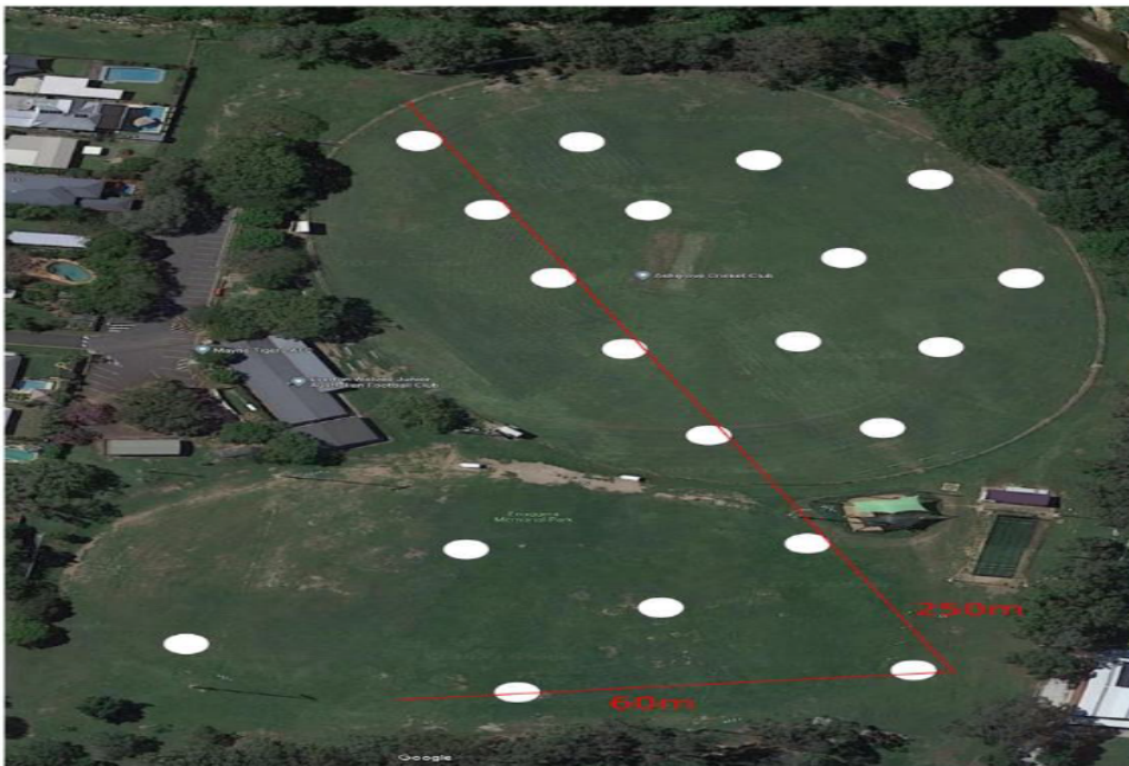
Figure 3 Aerial imagery illustrating the position and layout of Ground Control Point (GCP) targets (white circles, not to scale) utilized in this study
