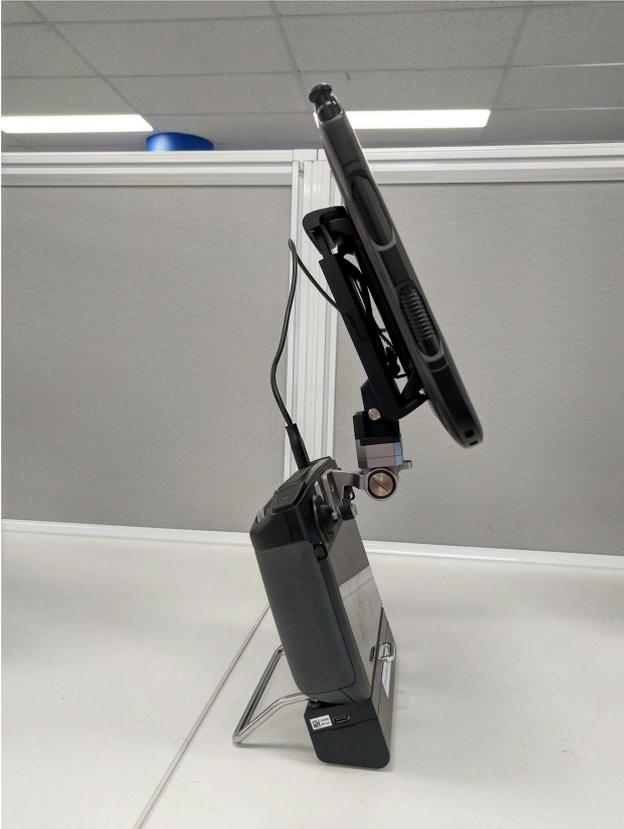
5. Connect the tablet to the controller using a USB cable.
