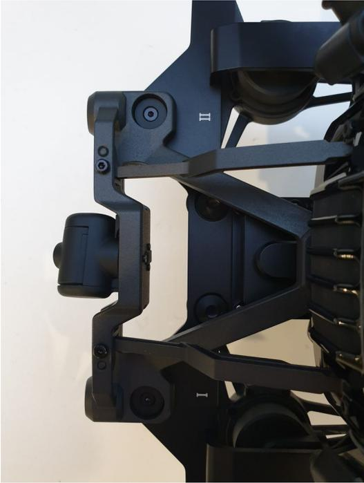
6. Remove the six PH#0 fasteners from inside both sides of the battery tray (three per side).
