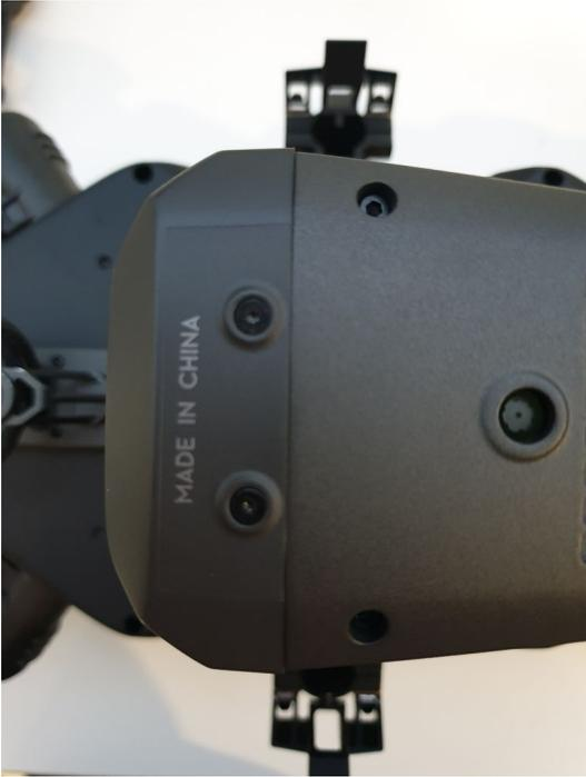
8. Remove the cover plate from the power distribution board (PDB) by pulling up and away from the drone.
