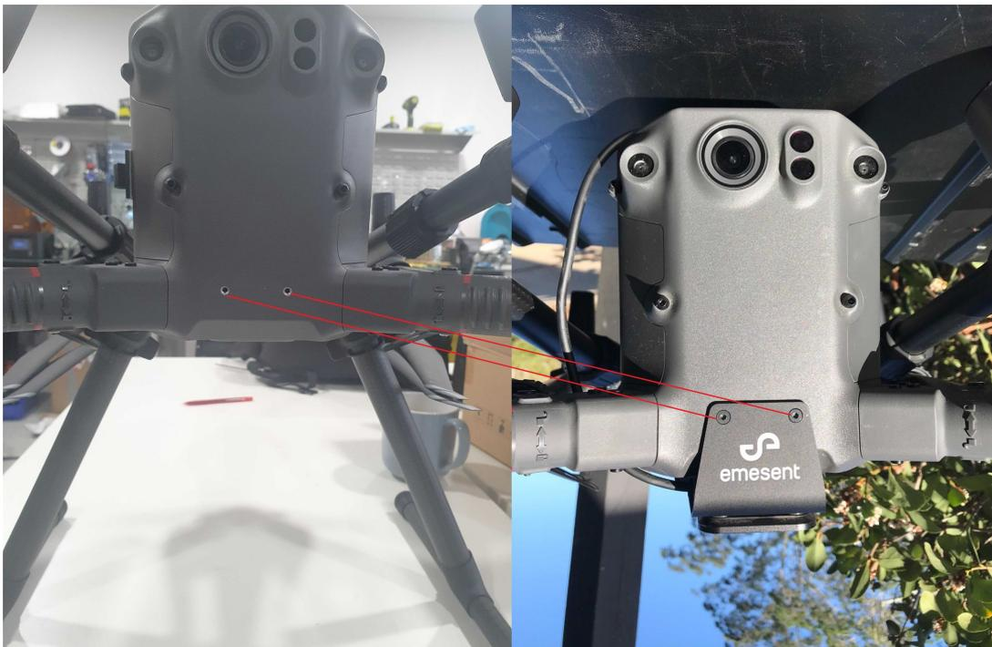
**Figure 2** DJI M300/M350 front mounting supports
