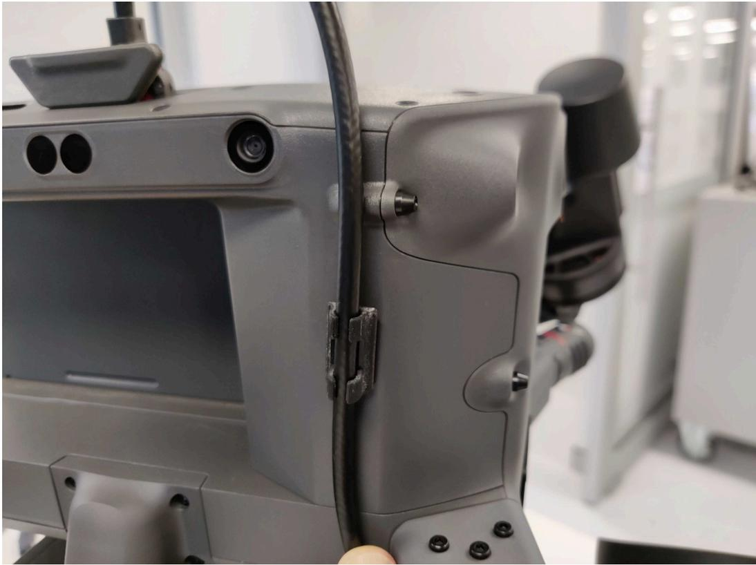
**Figure 5** Cable fixing and routing
