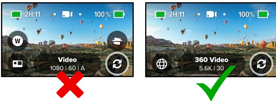
3. Once the GoPro MAX has been set to the correct mode and the Hovermap scan has started, press the red **Record** button on the top face of the GoPro MAX.
