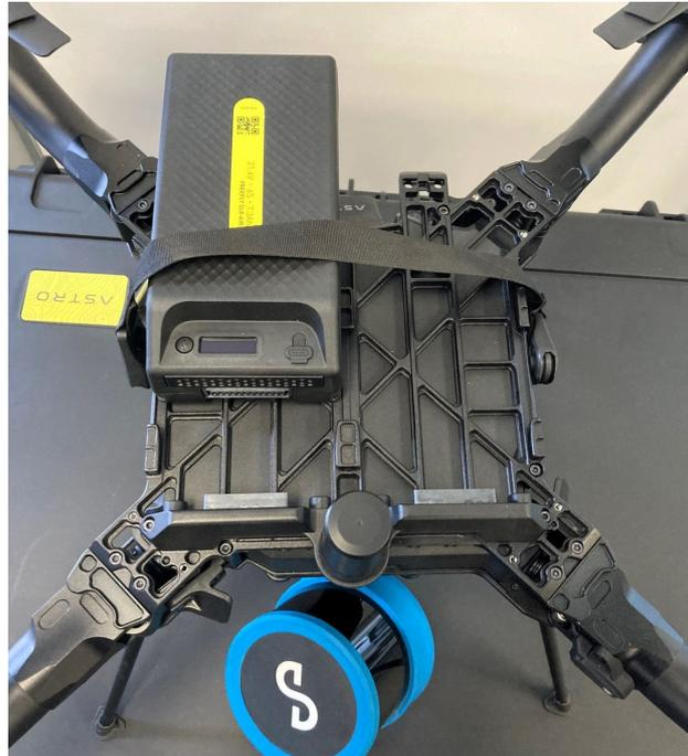
3. Press the power button on either of the batteries twice to power the aircraft.
