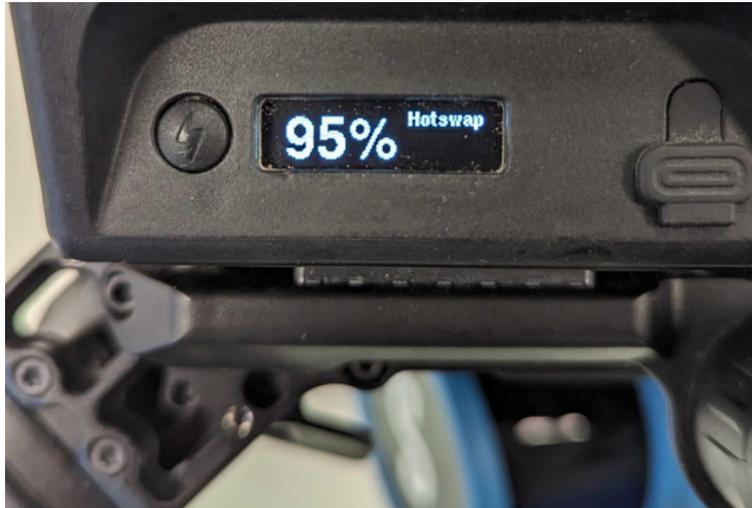
5. The second battery automatically powers up (and also shows "Hotswap" on the display) when the first battery is turned on. The green and red LEDs should light up at the end of the aircraft arms.
