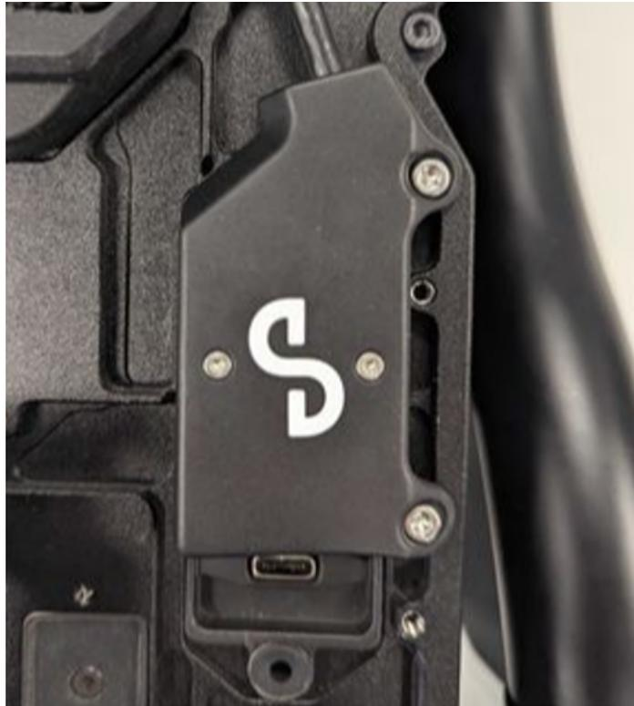
8. Insert the round end of the dust cover into the rubber grommet next to the USB-C port, and then connect the opposite end of the cover to the USB-C port.
