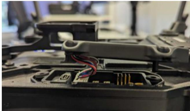
**i** Be careful not to crush the cables between Astro and the lip of the plastic cover.
