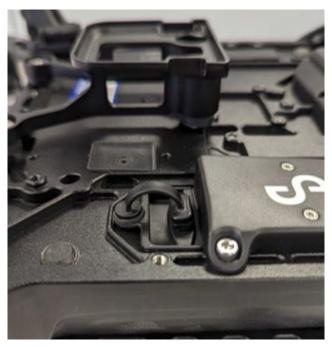
9. The following image shows the I/O shield properly secured and the USB-C dust cover in place. You can now proceed to turn the aircraft upright.
