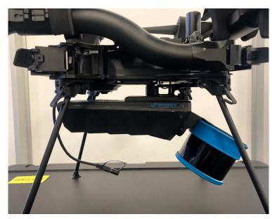
2. Align the white dot on the electrical interface with the white dot on the port on the Hovermap ST-X. Press firmly to connect the electrical interface, making sure it locks into place. A clicking sound indicates the cable has been successfully attached to the Hovermap ST-X.
