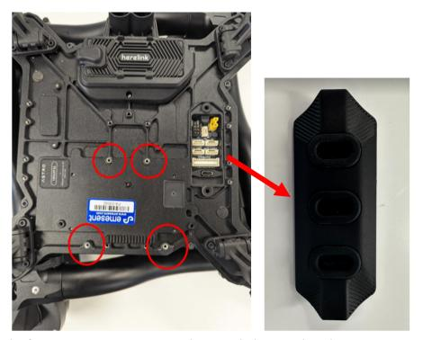
4. Screw in the four mounting screws using the provided 2.5mm hex driver.
