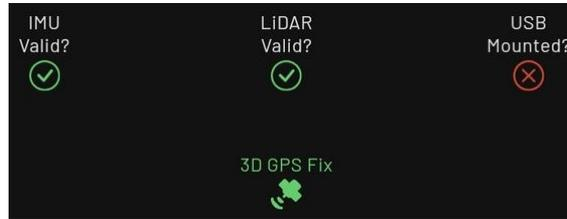
The Hovermap status icons show the status of the IMU, the LiDAR, and the USB connection.
