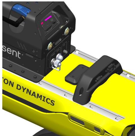
Figure 6 GXP position for when rear-mounted payloads are not required
