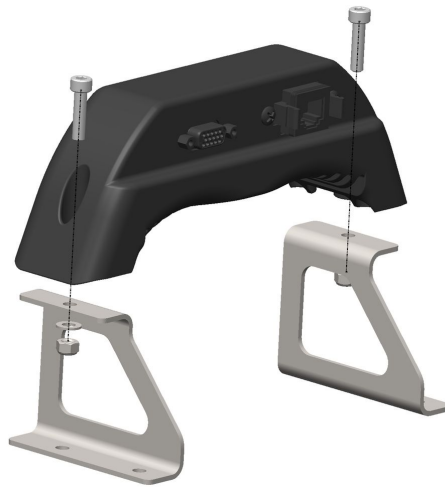
Figure 7 GXP attachment to the risers
