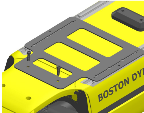
Figure 2 Alignment plate attachment to Spot
