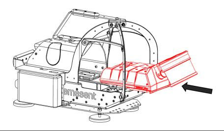
• Ensure that the two dovetail locks are secured.
