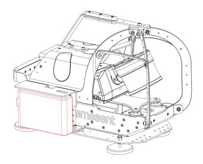
• The Hovermap is powered externally through an M12 connector.
